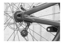
Carefully route the loose chain around the rear sprocket and hook it over the top guide pulley as shown in the 1st image.
