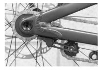
allow it to rest on the inner surface (next to the spokes). Untighten the axle bolts and slide out the wheel. The chain can be unhooked from the freewheel/rear sprocket and allowed to hang from the front sprocket once the hub is clear of the frame.
