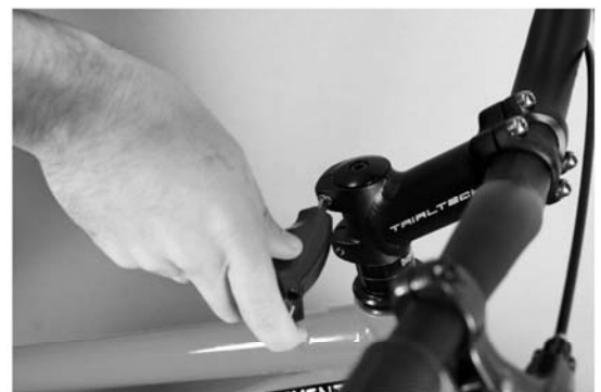
f) Loosen the stem bolts before adjusting the headset.
