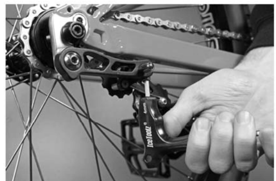
d) Chain tension can be adjusted by altering the cage position.
