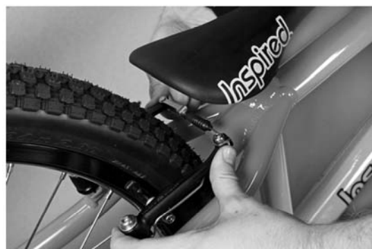
h) Push the brake arms together to release the noodle.
