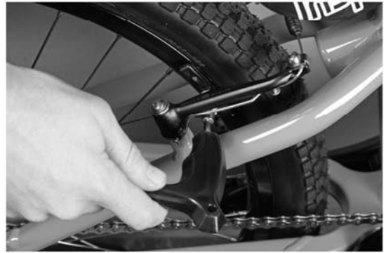
i) Ensure the brake pad contacts the rim correctly before tightening fully.
