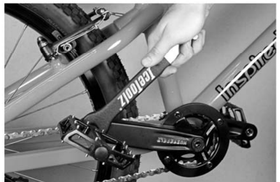
b) Tighten the pedals clockwise whilst holding the crank arm.
