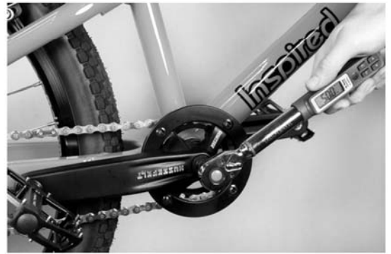
e) Keep the crank bolts tightened to the recommended level at all times.
