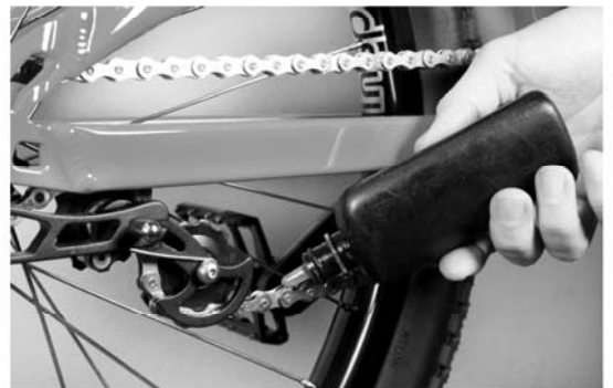
c) Apply a small amount of lubricant to the top of the chain.
