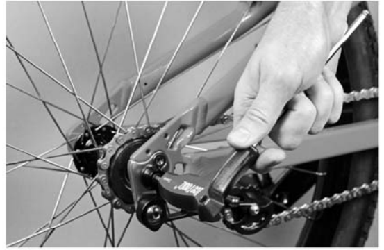
a) Check all wheel bolts/quick releases are tight before riding.
