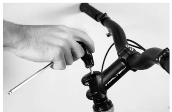
g) Tighten the top cap to remove play from the headset.
